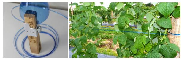
*Figure 20 – Bottlecutter. Source: www.plasticbottlecutter.com*
